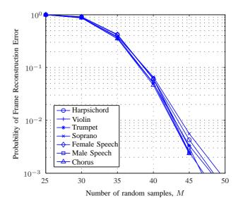
Fig. 6. Probability of frame reconstruction error vs the number of random samples for individual signals, with 4-bit quantization of the random samples, 3 bits for spectral whitening, and  $N_{\rm FM}=64$ .
