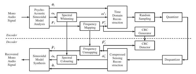
Fig. 1. A block diagram of the proposed system. In the encoder, the sinusoidal part of the monophonic audio signal is encoded by randomly sampling its time-domain representation, and then quantizing the random sample using scalar quantization.
