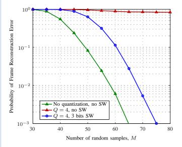
Fig. 2. Probability of frame reconstruction error vs the number of random samples per frame for three cases: no quantization and no spectral whitening, Q=4 bits quantization and no spectral whitening, and Q=4 bits quantization and 3 bits for spectral whitening.
