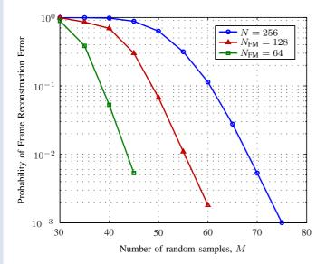
Fig. 4. Probability of frame reconstruction error *vs* the number of random samples per frame for various values of frequency mapping, with 4-bit quantization of the random samples, and 3 bits for spectral whitening.
