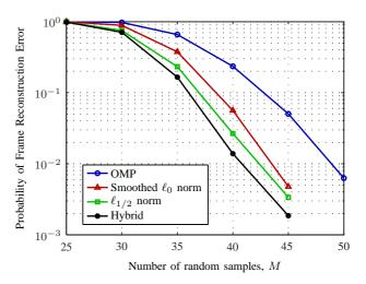
Fig. 5. Probability of frame reconstruction error vs the number of random samples per frame for different reconstruction algorithms, with 4-bit quantization of the random samples, 3 bits for spectral whitening, and  $N_{\rm FM}=64$ .
