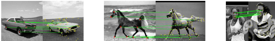
Fig. 8: Deformable feature matching via MRF optimization. From user selected features in a source image, we seek correspondences to automatically extracted features in a target image (feature similarity and geometric structure are both taken into account).
