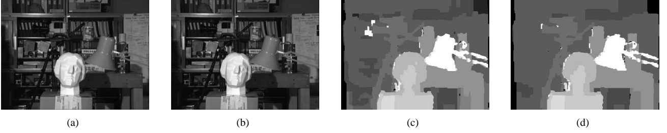
Fig. 7: (a) The left and (b) right images for one stereo pair from the Tsukuba data set. (c) The disparity estimated by the PD1 algorithm. (d) The corresponding disparity of the PD 2_{\mu=1} algorithm. This algorithm was shown to be equivalent to the expansion Graph Cuts algorithm. In both of the above cases the Potts metric has been used as the distance between labels. Since this distance is a metric the algorithms PD 3_a , PD 3_b , PD 3_c coincide with PD 2_{\mu=1} in this case and therefore produce the same result as that in figure (d).
