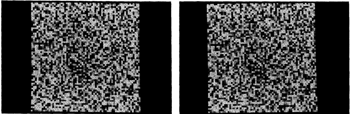
Fig. 3. The two frames of a test case used frequently in this work are displayed. The test frames contain a central square that is displaced one pixel to the right between FRAME-1 and FRAME-2. This frame pair does not contain added noise.
