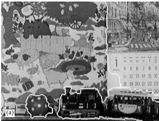
Fig. 6. ‘Mobile’ sequence. (a) Segmentation map obtained at time t_1 . (b) Enlargement of one part of the segmentation map obtained at time t_4 . \eta = 0.6 . We obtain similar results for values of \eta ranging from 0.4 to 1.5.
