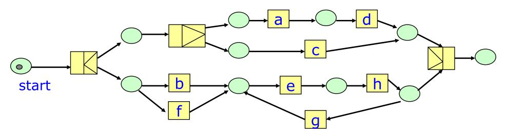
•The workflow net results from applying the patterns of the basic building blocks, hence it is safe and sound.
