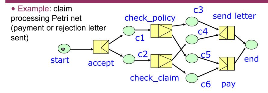
if a token is placed in c5 by transition check\_policy, and a token is placed in c6 by check\_claim, pay will fire (correct!)
