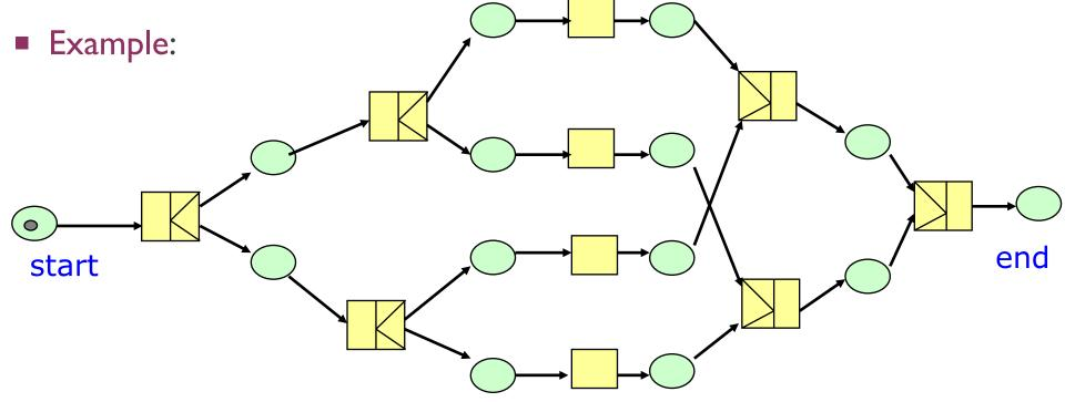
The two paths that originate at one AND-split should meet in the same AND-join.
