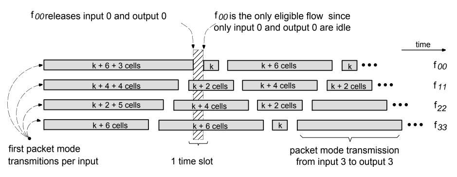
during the cell-time when a packet transmission is completed at an inputoutput pair, if this is the only input-output pair that gets released and there are more packets in that VOQ, then the same pair will get reconnected
