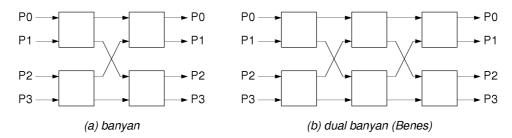
(b1) Network (b) consists of two banyans connected back-to-back, with their middle stages merged; this is a *Benes* network. Is this a single-path or multi-path network? How many different routes are there from a given input port to a given output port, for the different input-output port pairs (flows)?
