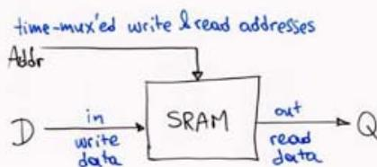
⊖: data path underutilization when imbalanced ( $\neq 50\% - 50\%$ ) read/write transactions
