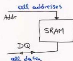
⊖: bus turn-around overhead: data bus underutilization when frequently switching between read & write transactions
