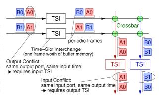
In §5.2, slide 11 (?) (also shown below on the right), we saw the 3-stage Clos network (and, before that, its specialization, the Benes network). There is an analogy --or even equivalence-- between these two systems in circuit switching (the analogy carries over to packet switching, with TST becoming an input-queued or CIOQ crossbar, and Clos becoming a "Parallel Packet Switch" (PPS)). The analogy goes as follows. Each of
