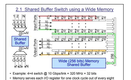
Note hidden input and output crossbars; note required cell time alignment
