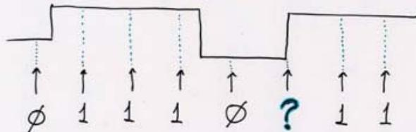
Since the signal changes asynchronously to the sampling clock, the sampling point "?" could have been a little before or a little after the signal changes, yielding either  $\emptyset$  or 1. Hence, it does not matter if the FF metastability eventually yields  $\emptyset$  or 1 - all that matters is that it becomes a valid binary value, that all of its receivers interpret in the same way.
