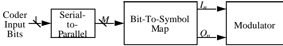
Figure 15 - Differential / Gray Coder Block Diagram
