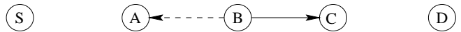
Figure 2: When B forwards a packet from S toward D through C, A can overhear B's transmission and can verify that B has attempted to pass the packet to C. The solid line represents the intended direction of the packet sent by B to C, while the dashed line indicates that A is within transmission range of B and can overhear the packet transfer.
