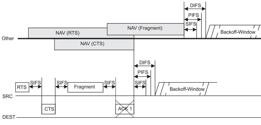
Figure 56—RTS/CTS with transmitter priority and missed acknowledgment
