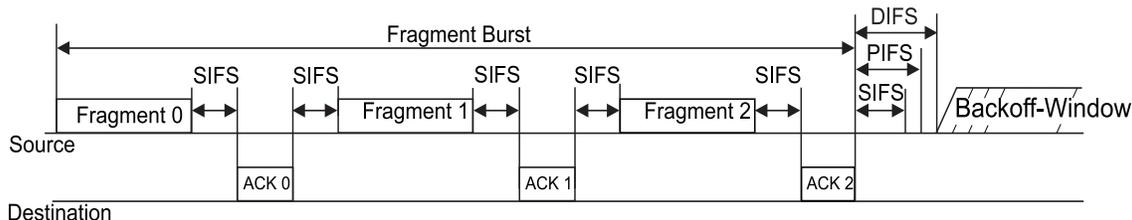
**Figure 54—Transmission of a multiple-fragment MSDU using SIFS**
