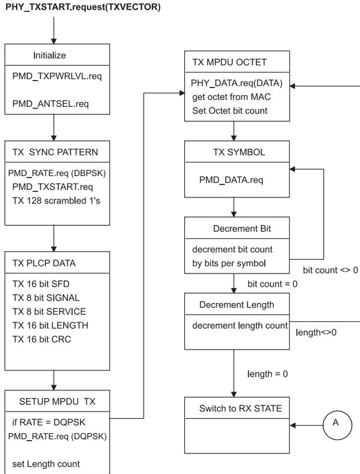
A At any stage in the above flow diagram, if a PHY\_THEND. Request is received.
