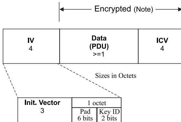
NOTE – The encypherment process has expanded the original Frame Body by 8 octets, 4 for the IV field and 4 for the ICV. The ICV is calculated on the data field only.
