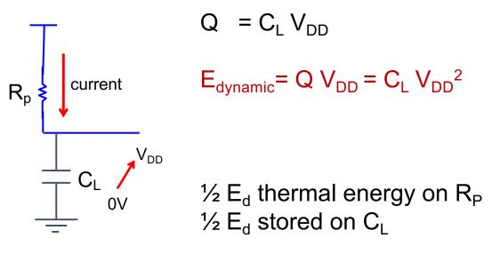
$$Q = C_L V_{DD}$$
