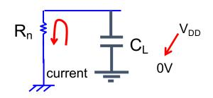
$\frac{1}{2}$  E<sub>dynamic</sub> stored on C<sub>L</sub> becomes thermal energy on R<sub>N</sub>
