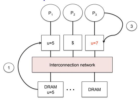
Processor 3 writes new value of *u*. Processor 1 and processor
