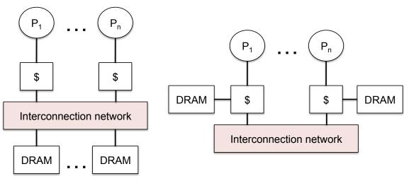
Though hardware classification based on physical placement of memory relative to processors, multiprocessors are classified also based on the abstraction of memory provided to users. Abstraction of memory is typically decoupled from the actual implementation.
