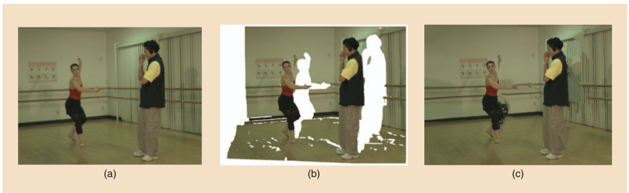
[FIG12] The view synthesis for the sequence ballet. (a) The known reference view projected into virtual viewpoints. (b) Projection of the reference view on a virtual viewpoint with rightward shift of the camera (white areas are disoccluded areas). (c) The inpainted version of the projected image. (Images used courtesy of [67].)
