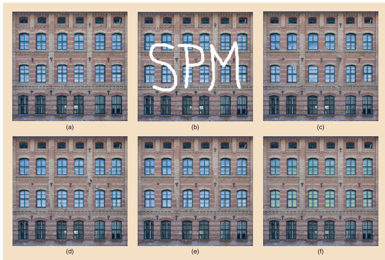
[FIG10] Image restoration. (a) The original image (courtesy of [62]), (b) mask, (c) inpainting results with anisotropic diffusion, (d) exemplar-based method with similarity weights (NLM), (e) with the hybrid method (courtesy of [21]), and (f) with the tensor completion technique (courtesy of [62]).
