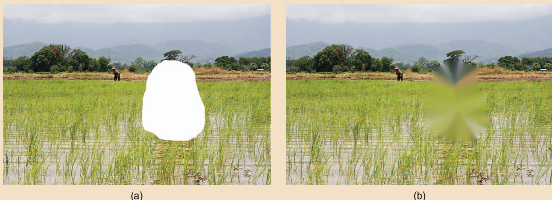
[FIG3] Typical blurring effects of (a) and (b) diffusion-based methods (example with the method in [10]) when the hole to be filled is large. [(a) courtesy of [39]. (b) generated by Christine Guillemot and Olivier Le Meur.]
