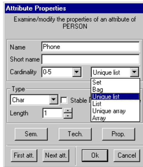
Figure 9.14 - Multivalued attributes can define mere sets. However, they can alternately form bags, lists, lists of unique values, arrays or arrays of distinct values.
