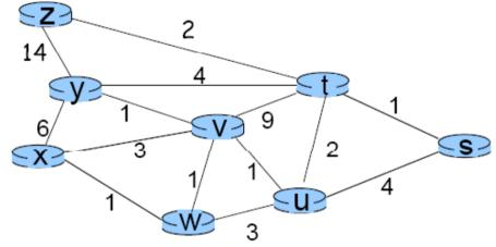
We can now build x's forwarding table. E.g. the entry to s will be constructed by looking at predecessors along shortest path: 6,t 5,u 3,v 2,w (direct link) So forward to s via w
