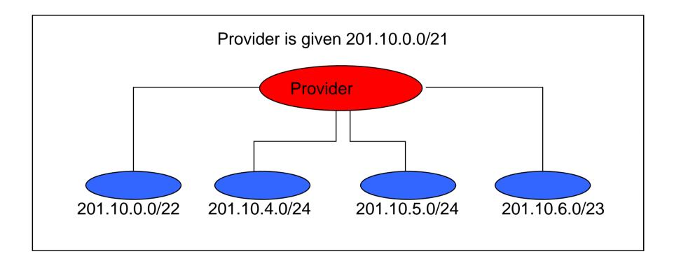
Routers in the rest of the Internet just need to know how to reach 201.10.0.0/21. The provider can direct the IP packets to the appropriate customer.
