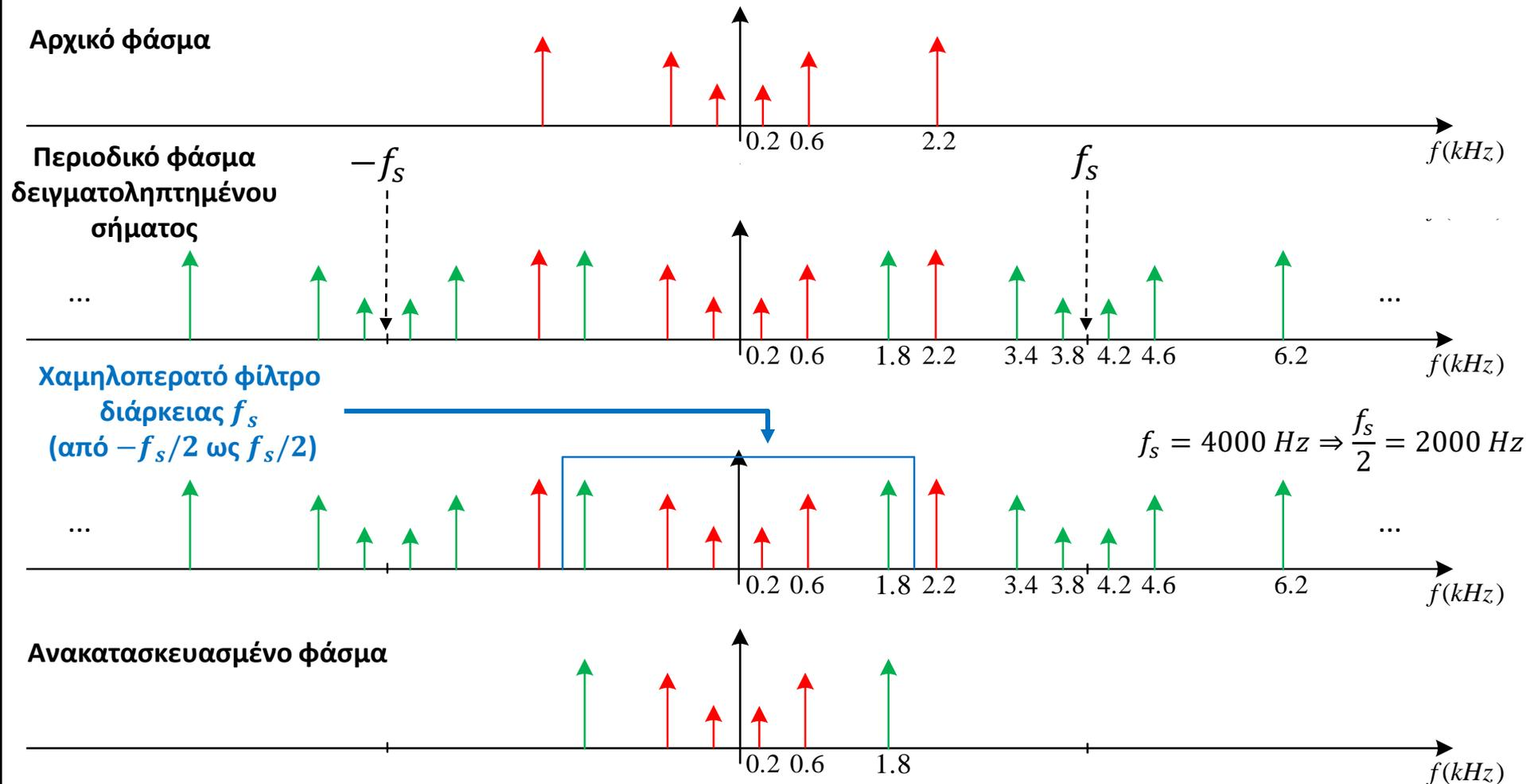
$$f_s = 4000 \text{ Hz} \Rightarrow \frac{f_s}{2} = 2000 \text{ Hz}$$
