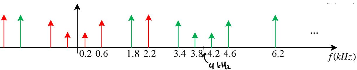
$$f_s = 4000 \text{ Hz} \Rightarrow \frac{f_s}{2} = 2000 \text{ Hz}$$
