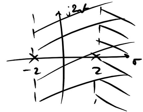
$$\Rightarrow Y(s) = H(s)X(s) = \frac{1}{(s-2)(s+1)(s+2)}, \quad R_Y = R_X \cap R_H = \{\sigma > 2\} \cap \{\sigma > -2\} = \sigma > 2.$$
