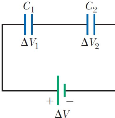
$$\frac{1}{C_{\text{eq}}} = \frac{1}{C_1} + \frac{1}{C_2}$$
