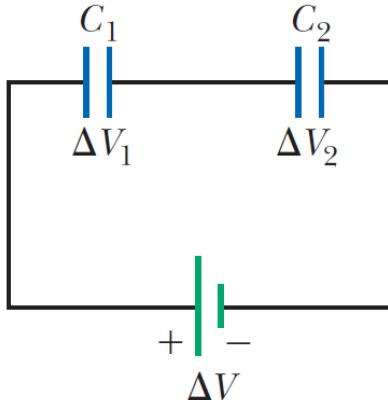
$$\frac{1}{C_{\text{eq}}} = \frac{1}{C_1} + \frac{1}{C_2}$$
