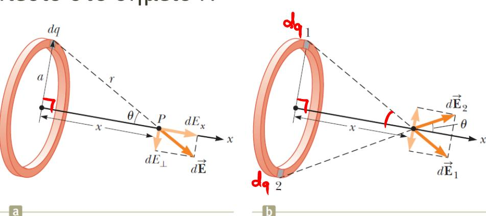
$$dE_x : dE_x = k_e \frac{dq}{r^2} \cdot \cos\theta \quad \left. \begin{aligned} r^2 &= a^2 + x^2 \\ \cos\theta &= x/r \\ r &= \sqrt{a^2 + x^2} \end{aligned} \right\} \Rightarrow dE_x = k_e \frac{dq}{a^2 + x^2} \cdot \frac{x}{\sqrt{a^2 + x^2}}$$
