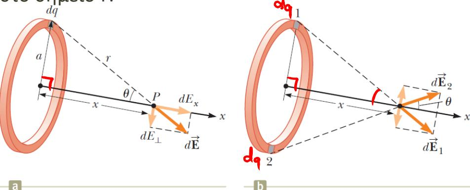
$$dE_x : dE_x = k_e \frac{dq}{r^2} \cdot \cos\theta \quad r^2 = a^2 + x^2 \quad \left. \begin{array}{l} dE_x = k_e \frac{dq}{a^2+x^2} \cdot \cos\theta \\ \cos\theta = x/r \\ r = \sqrt{a^2+x^2} \end{array} \right\} \Rightarrow dE_x = k_e \frac{dq}{a^2+x^2} \frac{x}{\sqrt{a^2+x^2}}$$
