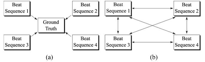
Fig. 1. Setups for determining difficulty of a sample for  $N = 4$  beat trackers. (a) With and, (b) Without ground truth (a) Ground truth given (b) No ground truth.
