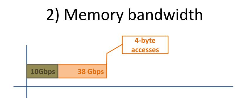
• Packet reading is boosted 4x with 4-byte fetches
