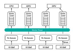
Fig. 3. Pythia architecture for processing network packets.
