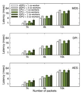
Fig. 2. Overall latency for processing 1500-bytes network packets.
