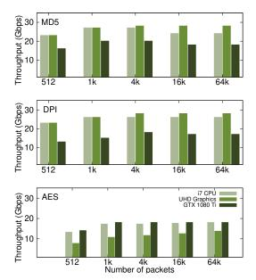
Fig. 1. Throughput sustained for processing 1500-bytes network packets.
