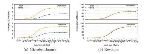
Fig. 3: Throughput comparison between the AES-128 CTR found in Android's Keystore and the SGX-enabled version provided by Andromeda's Keystore.
