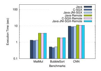
Fig. 5: Performance comparison of the different Andromeda-enabled execution methods, including offloading, against the vanilla Java versions.
