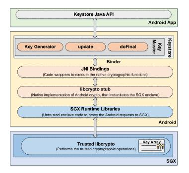
Fig. 2: The Keystore Architecture. The cipher keys are stored only in SGX enclaves. Developers can encrypt and decrypt their data using the default Keystore API, which internally redirects to Andromeda's trusted implementation.
