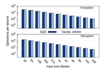
Fig. 4: Sustained throughput achieved for the vanilla and the SGX-enabled implementation of the RSA-1024 cryptographic algorithm.
