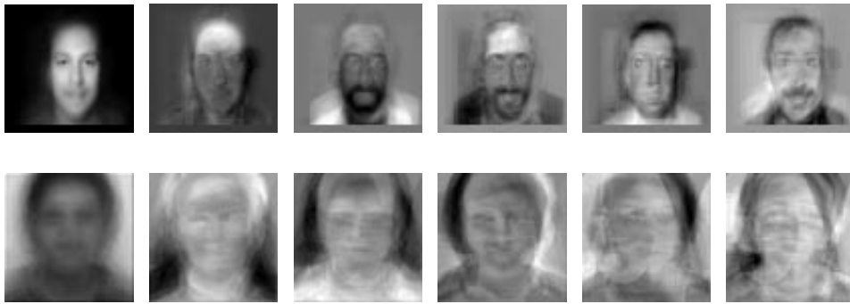
Fig. 10. The first 6 eigenfaces of the FACES database (first line) and the FERET database (second line)
