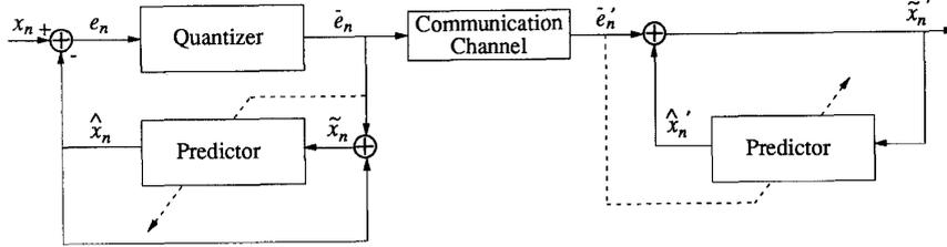
fig. 2.1: Structure of the ADPCM system
