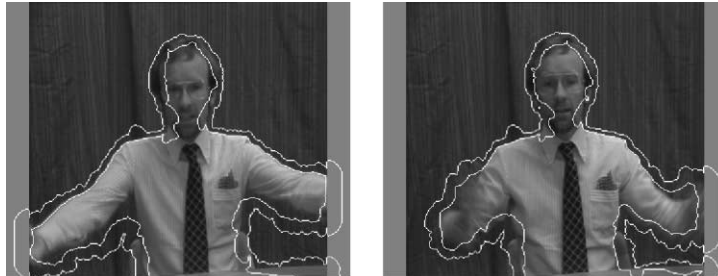
Fig. 7. Extraction of the uncertainty area on two frames of the Trevor White sequence.
