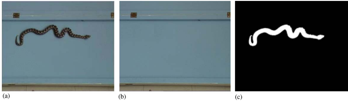
Fig. 8. (a) A snake image; (b) its background image; and (c) the extracted snake silhouette.
