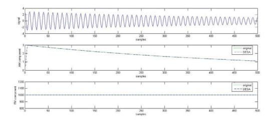
Figure 3.5: Separation into its components for an AM signal  $x(t) = Ae^{-at}cos(2\pi f_r t)$
