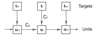
Figure 1.4: Target cost and concatenation cost. Target cost measures the closeness between target,  $t_i$ , and unit,  $u_i$ . Concatenation cost measures the continuity between previous unit,  $u_{i-1}$ , and current unit,  $u_i$ .
