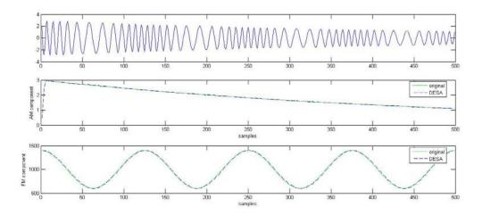
Figure 3.7: Separation into its components for an AM&FM signal  $x(t) = Ae^{-at}cos(2\pi f_r t + \beta sin(2\pi f_m t))$
