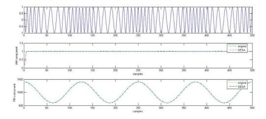
Figure 3.6: Separation into its components for an FM signal  $x(t) = cos(2\pi f_r t + \beta sin(2\pi f_m t))$
