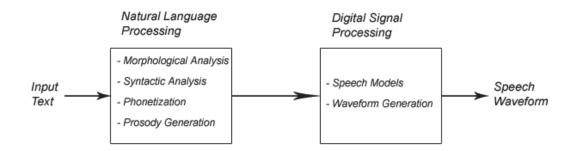
Figure 1.2: Modules of a Text-to-Speech Synthesis System. In order to produce high quality synthesized speech, experts from different fields should collaborate.
