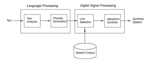
Figure 1.3: Modules of a Unit Selection Synthesis System.
