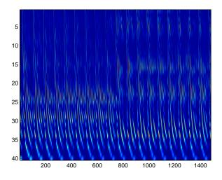
Figure 3.10: Cochleagram from a synthesized speech segment. In the middle of the segment, the concatenation point is evident.
