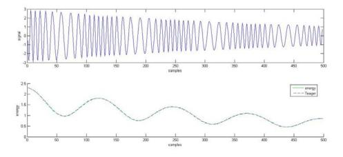
Figure 3.4: Energy of an AM&FM modulation signal. We consider as instant energy the product of instant amplitude and instant frequency. Observe the peaks of energy when signal oscillates faster and the valleys when signal oscillates slowly.
