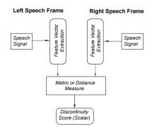
Figure 1.6: Flow diagram for measuring the discontinuity of two successive speech units. meaningful physical interpretations.
