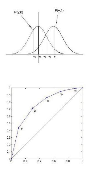
Figure 6.3: Receiver operator characteristic curve.  $P_D$  and  $P_{FA}$  are computed for various values of the threshold,  $\gamma$ .
