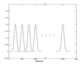
Figure 3.8: Filterbank of Gabor filters. These filters are equally spaced in frequency and they are slightly overlapping.
