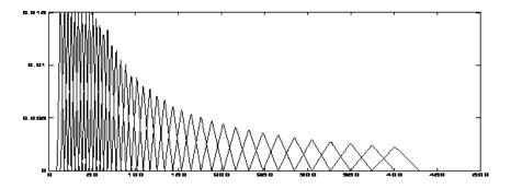
Figure 3.3: Filters of the filterbank. They are defined from the mel-scaled frequencies.
