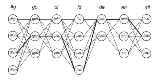
Figure 1.5: Candidate units constitute a k-partite graph. Each vertex has a weight which is the sum of target cost and concatenation cost. The shortest path is specified through Viterbi search algorithm. Here, best sequence of word *golden*, which is segmented into diphones, is found.
