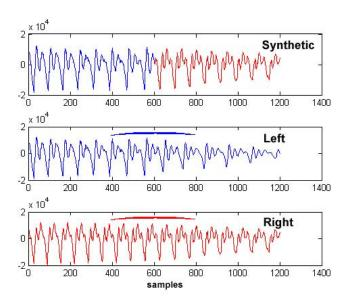
Figure 5.2: Where the analysis is done for the database of AT&T. First subplot shows the synthetic speech signal, while, the other two show the left and right speech segments.
