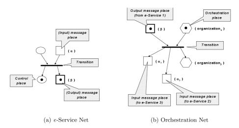
Fig. 2. Basic elements of the Petri Net-based model
