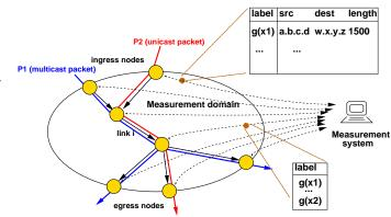
Fig. 1: SCHEMATIC REPRESENTATION OF TRAJECTORY SAMPLING. A measurement system collects packet *labels* from all the links within the domain. Labels are only collected from a pseudo-random subset of all the packets traversing the domain. Both the decision whether to sample a packet or not, and the packet label, are a function of the packet's invariant content.
