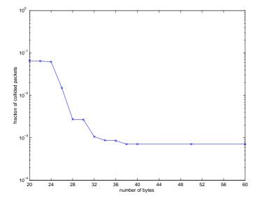
Fig. 4: PACKET COLLISIONS. The fraction of packets whose prefix is not unique, as a function of the prefix length l. The smallest value for the prefix length (20 bytes) corresponds to using only the packet header.
