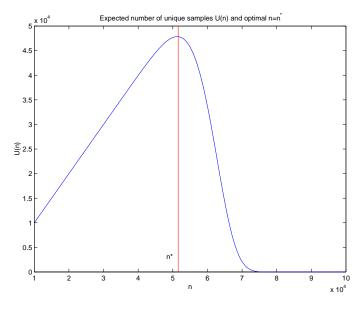
**Fig. 7:** THE EXPECTED NUMBER OF UNIQUE SAMPLES U(n) AS A FUNCTION OF n, FOR  $c = 10^6$  BIT. The optimal number of samples  $n^*$  is approximately  $5.15 \cdot 10^4$ , with  $m^*=19.4$  bit per label. The collision probability  $p_{coll}$  is approximately 0.072, i.e., 7.2% of the samples transmitted to the collection system have to be discarded.
