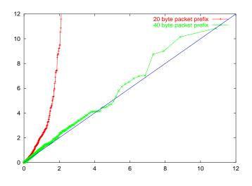
**Fig. 6:** HASH-SAMPLED ADDRESS BITS DISTRIBUTIONS. Quantile-quantile plot of address bit chi-square values vs. chi-squared distribution with 1 degree of freedom; for various traces, primes A, thinning factors r/A; see text. Close agreement for 40 byte packet prefixes; marked disagreement for 20 byte packet prefixes (i.e. no payload included for sampling hash)
