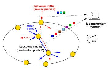
Fig. 8: MEASUREMENT EXPERIMENT. A simple experiment where labels from two links are compared to estimate what fraction of traffic on the backbone link comes from the customer access link.
