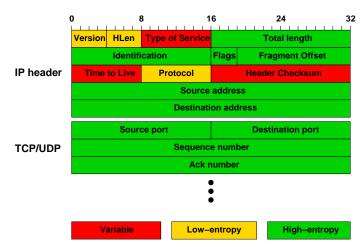
Fig. 2: INVARIANT PACKET CONTENT. The hash functions are computed over a subset of header fields and part of the payload. Variable field change along the path; low entropy fields are invariant along paths but vary little between packets; high entropy fields and invariant along paths and vary significantly between packets.
