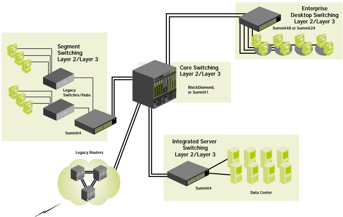
Figure 3: Extreme Networks' complete end-to-end systems solution covers the full spectrum, from redundant, fault-tolerant carrier-class chassis to high-density, low-cost desktop switching.
