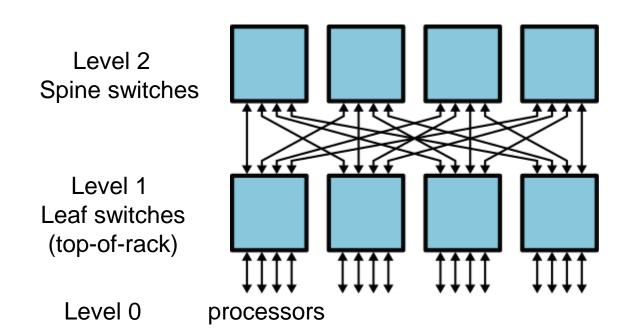
Spine nodes are the roots of the fat tree, and leaf nodes are the switches at height 1 – in k-ary ntree terminology, leaf nodes are the processors
