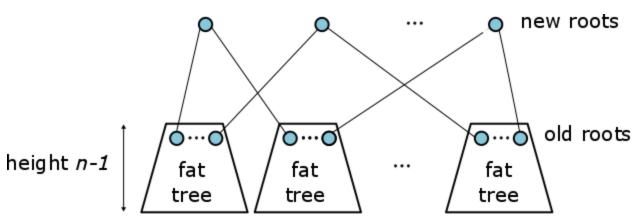
If we have a set of (sub) fat trees of height *n*-1 and we *arbitrarily* connect their roots to a set of a new (vertices) roots → fat-tree of height *n*
