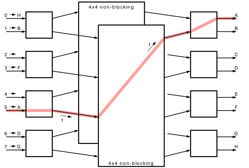
• Circuit Connections: Start from an input, use one of the subnets
