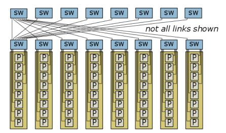
Global links implemented w. expensive optical links (electronic cables < 10 meter)
