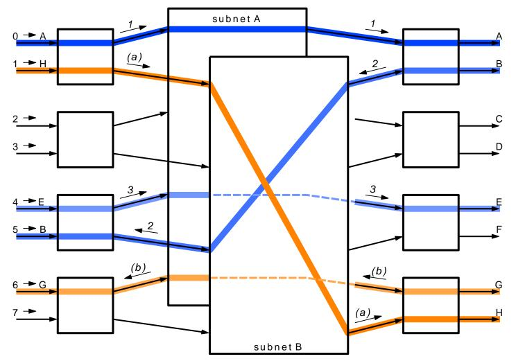
• New threads always start from a half-covered input switch, if there is one  $\Rightarrow$  all threads cover all out-sw's they touch, in-sw's are covered in sequence 5.2 - U.Crete - M. Katevenis - CS-534
