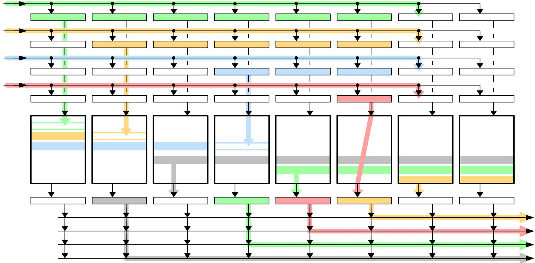
Ref: Katevenis, Vatsolaki, Efthymiou: "Pipelined Memory Shared Buffer for VLSI Switches", ACM SIGCOMM Conf. 1995, [http://archvlsi.ics.forth.gr/sw\\_arch/pipeMem.html](http://archvlsi.ics.forth.gr/sw_arch/pipeMem.html)
