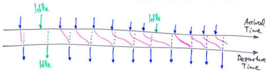
and/or  $\beta \Rightarrow$  notify the transmitter, by feedback ("backpressure") to slow-down or wait, i.e. to insert more idle's (so that they can be removed) ...
