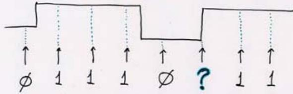
Since the signal changes asynchronously to the sampling clock, the sampling point "?" could have been a little before or a little after the signal changes, yielding either 0 or 1. Hence, it does not matter if the FF metastability eventually yields 0 or 1 - all that matters is that it becomes a valid binary value, that all of its receivers interpret in the same way.
