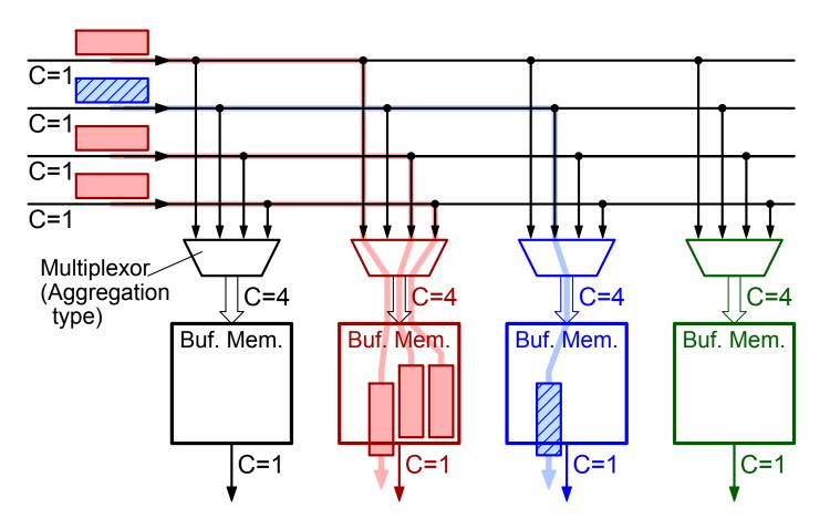
Memories are needed to temporarily buffer packets that cannot proceed due to (hopefully short-term) output contention
