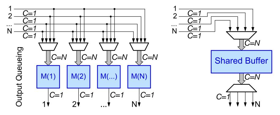
+ Aggregate memory throughput =  $2 \cdot N$ , versus  $N \cdot (N+1) = N^2 + N$  for Outp.Q
