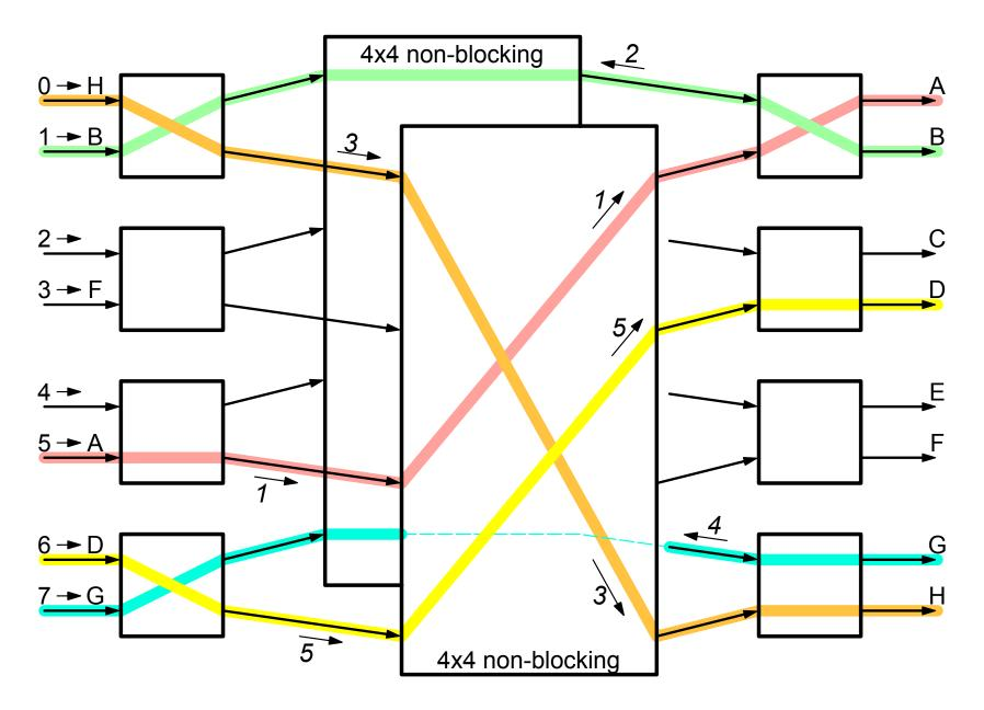
Keep "threading" output and input switches, till closing or no-connection
