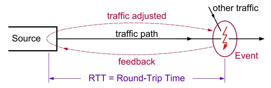
Traffic is "blind" during a time interval of RTT:
