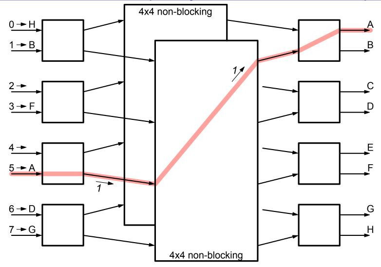
• Circuit Connections: Start from an input, use one of the subnets
