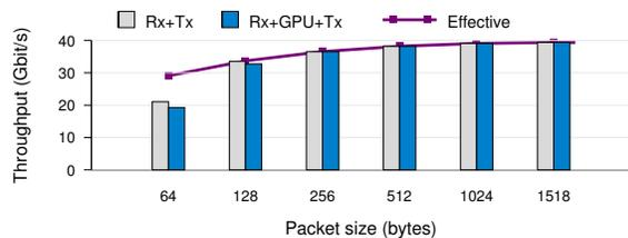
Figure 8: Data transfer throughput for different packet sizes when using two dual-port 10GbE NICs.
