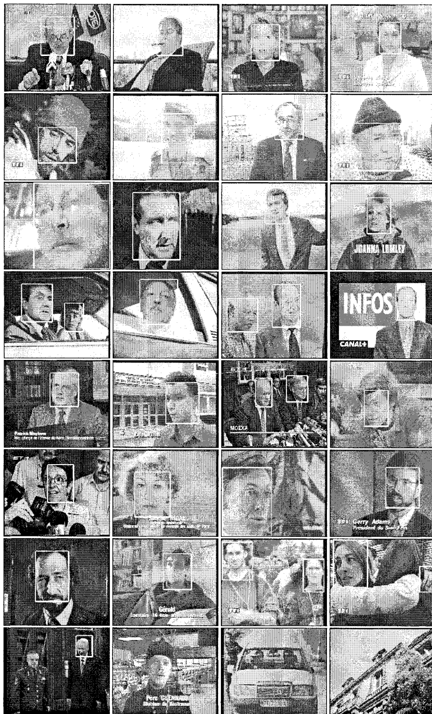
Fig. 9. Some detection results of our method for a subset of the test data set.
