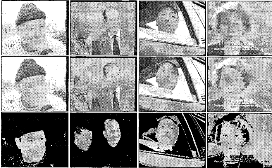
Fig. 3. Original images (first line), color quantized images (second line), and skin color filtered images (third line).
