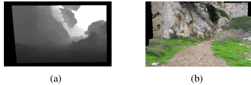
Fig. 1: (a) Depth map Z_0 of a local model (black pixels do not belong to its valid region dom_0 ). (b) A rendered view of the local model using an underlying triangle mesh
