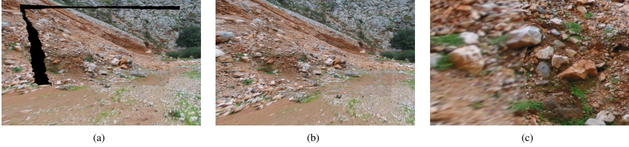
Fig. 5: Rendered views of the morphable 3D-model during transition from the key-position corresponding to image 2(a) to the key-position of image 2(b): (a) when no geometric morphing is applied to points in \bar{\Psi} and (b) when geometric morphing is applied to points in \bar{\Psi} . (c) A close-up view of the rendered image in (b). Although there is no geometric discontinuity, there is a difference in texture resolution between the left part of the image (points in \bar{\Psi} ) and the right part (points in \Psi ) because only points of the latter part are morphed photometrically.
