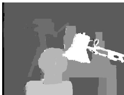
Fig. 17: Disparity for the “Tsukuba” image as estimated by the Fast-PD algorithm in the case where a Potts function has been used for the distance d(\cdot, \cdot) .
