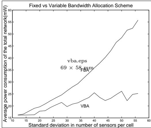
Fig. 5. Power consumption for different frequency allocation schemes
