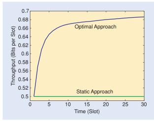
[FIG5] Spectrum opportunity tracking: A sequential decisionmaking problem where the throughput of secondary users improves over time due to accumulated observations.
