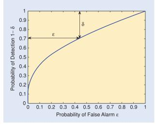
[FIG4] Receiver operating characteristics of spectrum opportunity detector.
