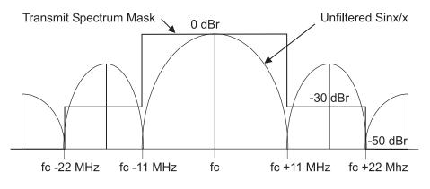
Figure 96—Transmit spectrum mask
