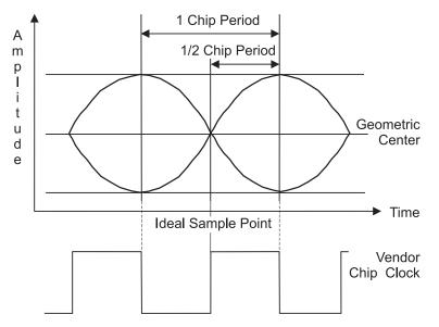
Figure 100—Chip clock alignment with baseband eye pattern
