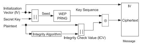
Figure 44—WEP encipherment block diagram
