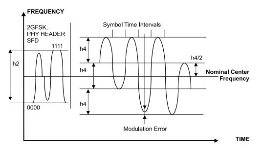
Figure 85—Four-Level GFSK transmit modulation
