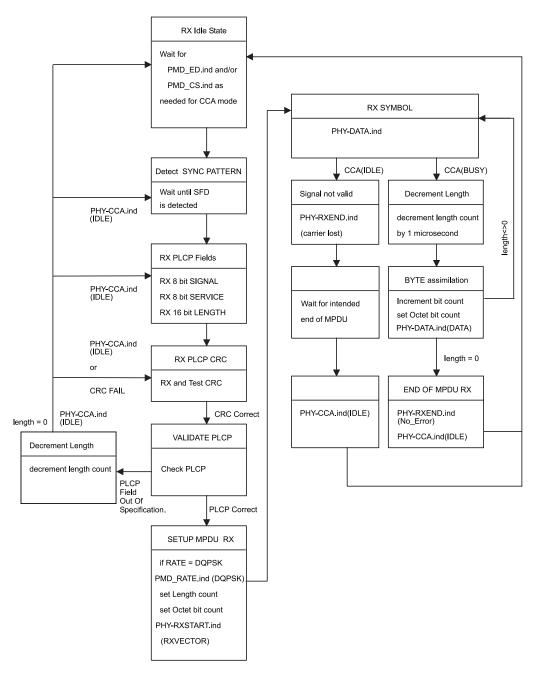
Figure 94—PLCP receive state machine
