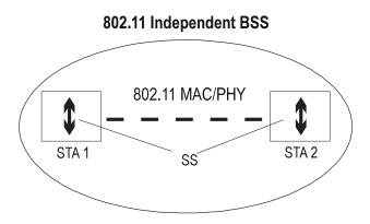
Figure 10—Logical architecture of an IBSS
