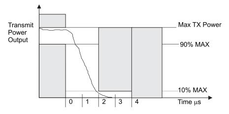
Figure 98—Transmit power-down ramp
