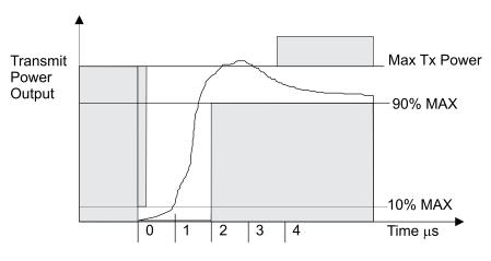
Figure 97—Transmit power-on ramp
