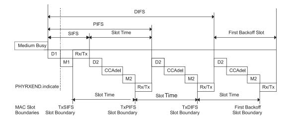
D1 = aRxRFDelay + aRxPLCPDelay (referenced from the end of the last symbol of a frame on the medium) D2 = D1 + Air Propagation Time Rx/Tx = aRXTXTurnaroundTime (begins with a PHYTXSTART.request) M1 = M2 = aMACPrcDelay CCAdel = aCCA Time - D1
