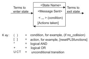
Figure 69—State diagram notation example
