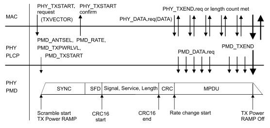
Figure 91—PLCP transmit procedure
