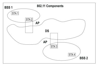
Figure 2 adds the DS and AP components to the IEEE 802.11 architecture picture.
