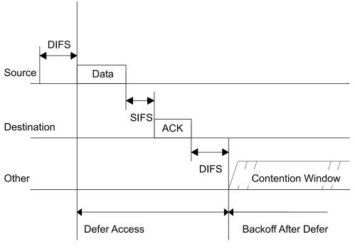
Figure 57—Directed data/ACK MPDU
