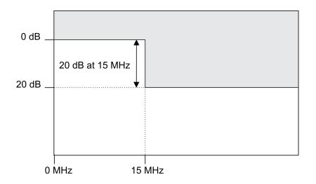
Figure 106—Transmit spectrum mask
