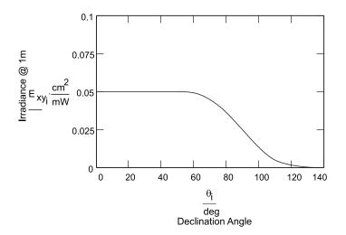
Figure 105—Emitter radiation pattern mask 2
