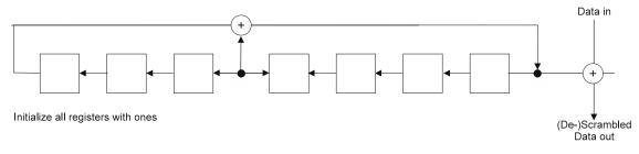
Figure 71—Frame synchronous scrambler/descrambler
