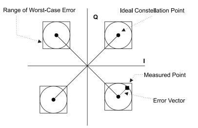
Figure 99—Modulation accuracy measurement example
