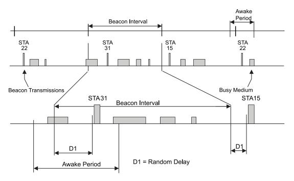
Figure 65—Beacon transmission in an IBSS
