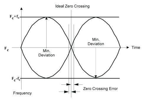
Figure 84—Transmit modulation mask
