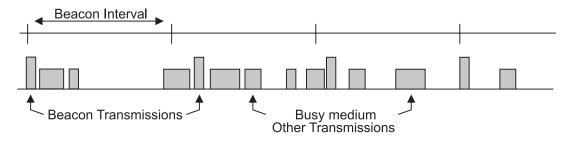
Figure 64—Beacon transmission on a busy network
