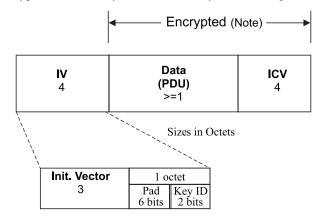
NOTE – The encypherment process has expanded the original Frame Body by 8 octets, 4 for the IV field and 4 for the ICV. The ICV is calculated on the data field only.
