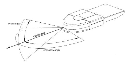
Figure 104—Mask 2 device orientation drawing
