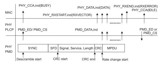
Figure 93—PLCP receive procedure
