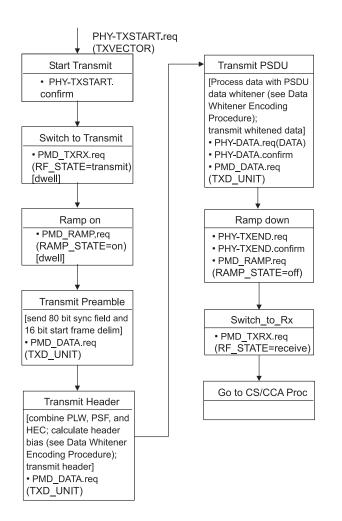
Figure 74—Transmit state machine
