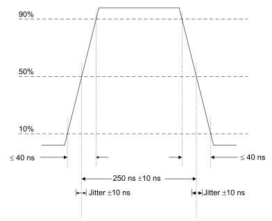
Figure 102—Basic pulse shape
