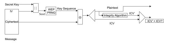
Figure 45—WEP decipherment block diagram
