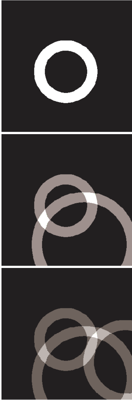
Fig. 2.10. An example of accumulation of votes on grid cells of a host at different time steps. The brighter an area, the more voting weight has been accumulated on the corresponding grid cells. The brightest area corresponds to a potential solution. The grid cell is too small to be distinguishable.
